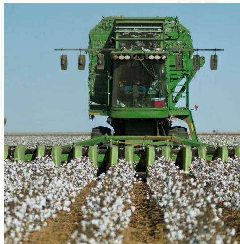
Cotton harvesters rely on cartridge valving for efficient control of the picking and cotton stripping operations.
